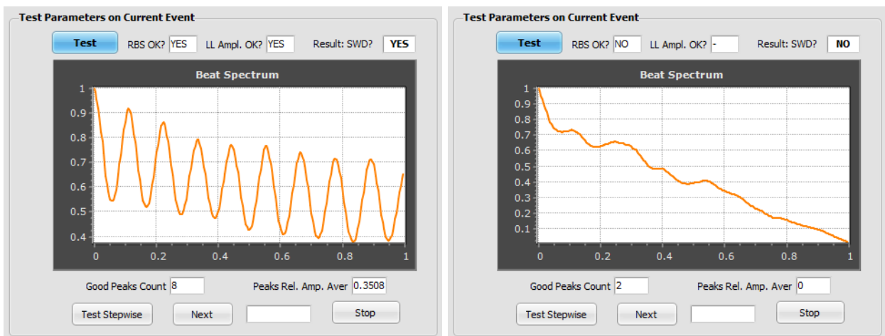
Fig. 1.6.15. Examples of the "Test Parameters on Current Event" widget look in case of processing an event that is a SWD (left) and of an event that is not (right).
